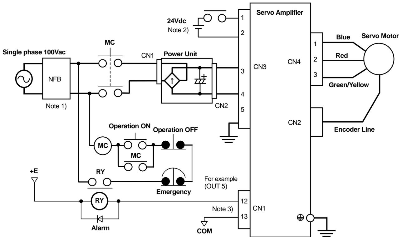
Note 1) It is recommended that an UL-approved earth leakage breaker be used that complies with IEC or EN standard.
