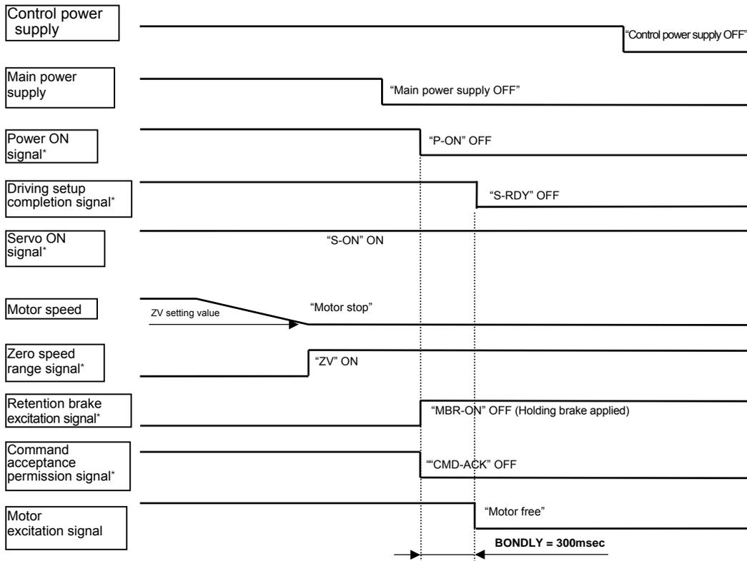
In the case of the model number: TS1B\*(50Vdc input type)
