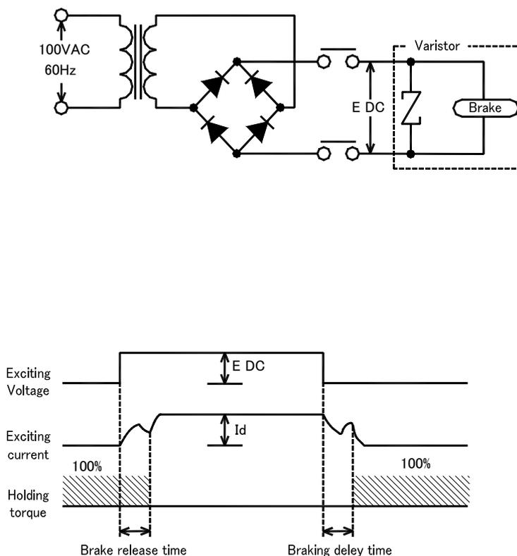
The brake release time and braking delay time refer to those mentioned in the above tables.
