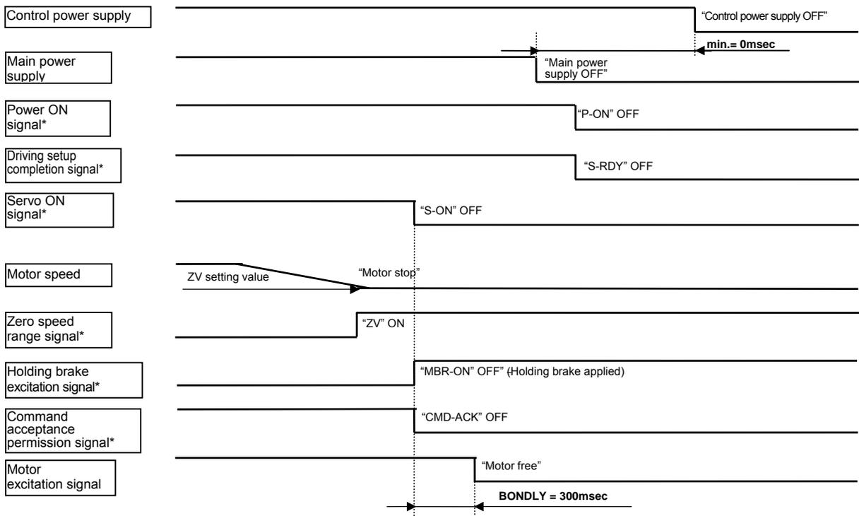
In the case of the model number: TS1B\*(50Vdc input type)
