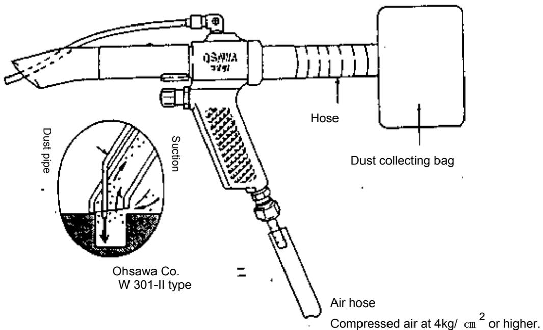
Fig.12 Example of a dust collector. (an inhale type)
