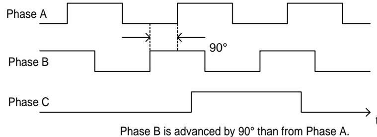
When the C-Phase is high, both A- and B- Phases cross the low level, once every revolution.
