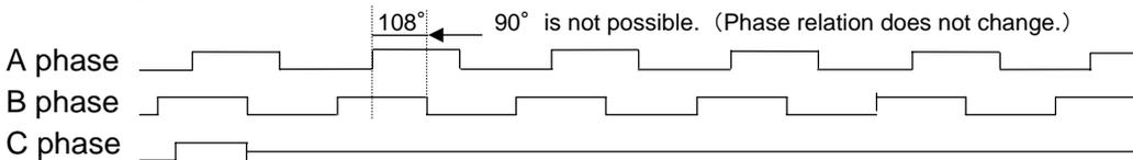
\* Destabilizes for 0.2 sec after control power is supplied.
