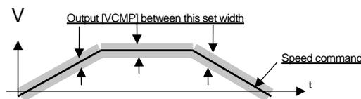
Speed transport settings: Speed transport signal is given if speed exceeds the set value.
