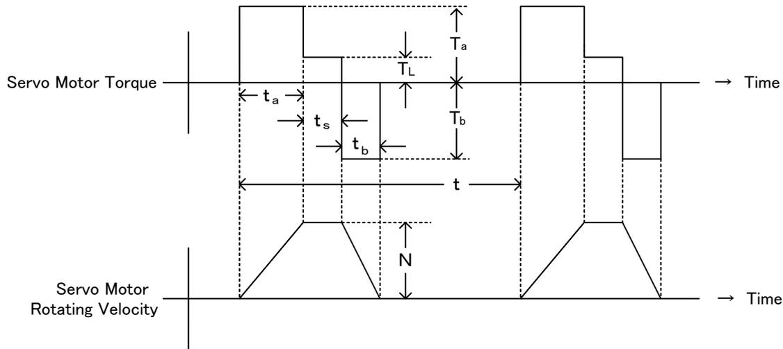
If the operating cycle is considered as 't', the usable range can be determined as follows:
