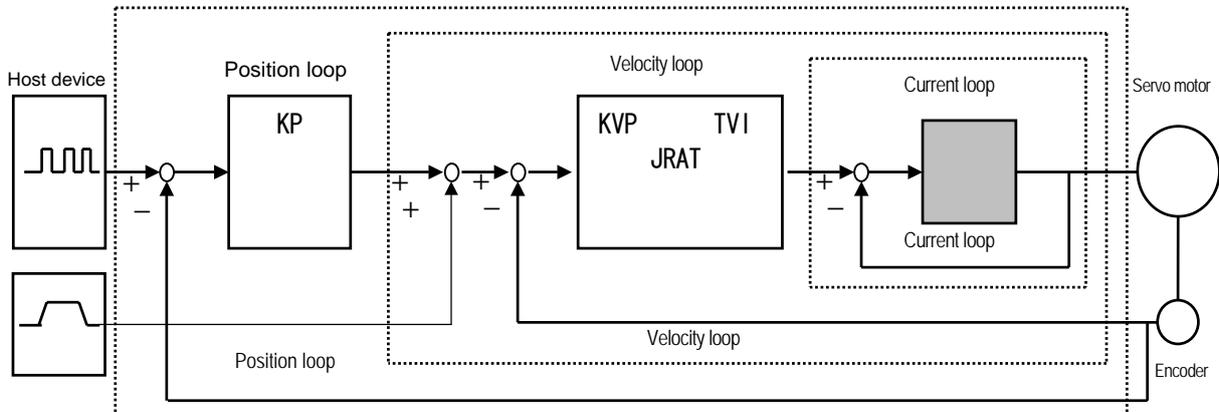
The response of the current loop is ensured internally in the servo amplifier, there is no need for the user to make additional adjustments.
