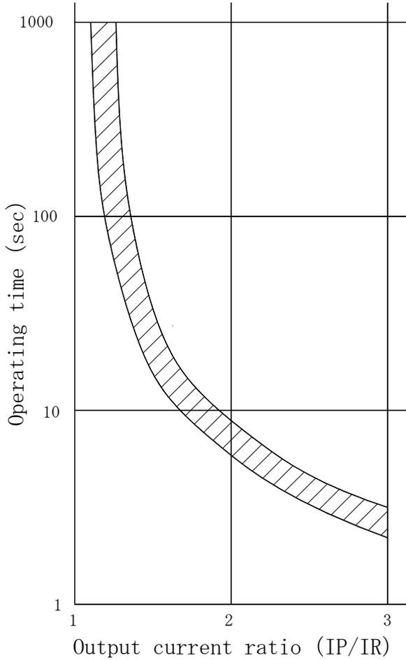
Overload characteristics of the T506 and down.
