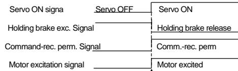
If there is a delay between the motor start and the holding brake release, that would be a brake failure as the motor operates with the holding brake on.
