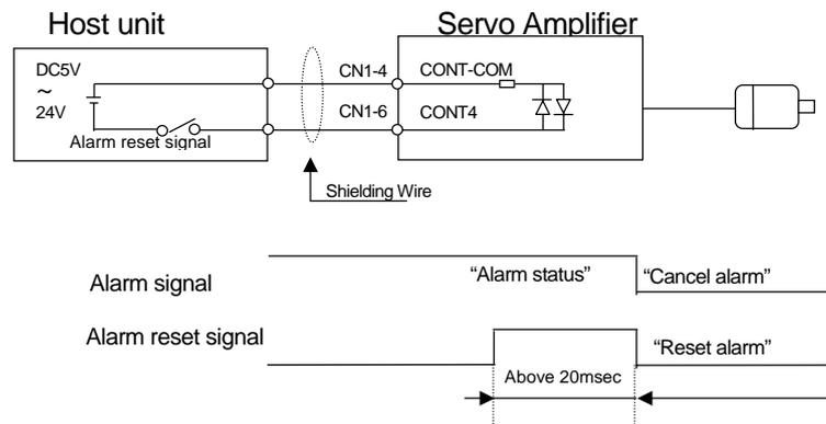
\* Note that any alarm not cleared by simply turning OFF the control power supply cannot be cleared with the alarm reset signal.
