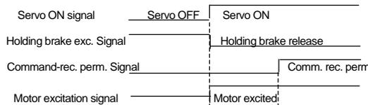
To extend the time period for a command acceptance controls time lag to prevent a holding brake from breakage.
