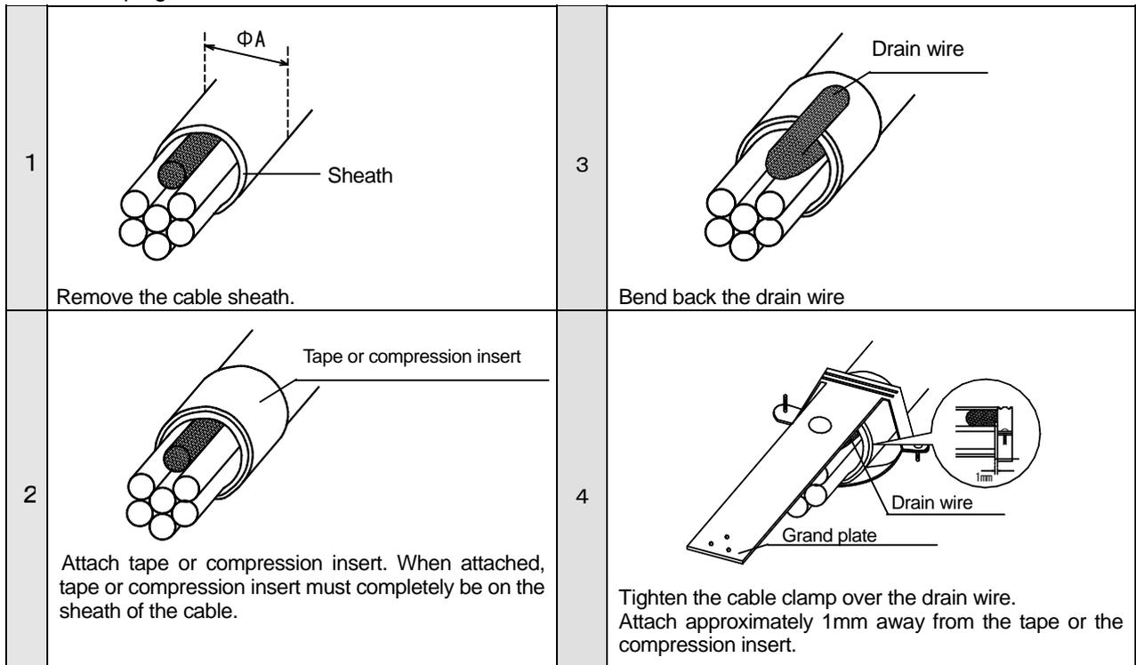
\* Compression insert should only be attached before soldering the cable to the connector
