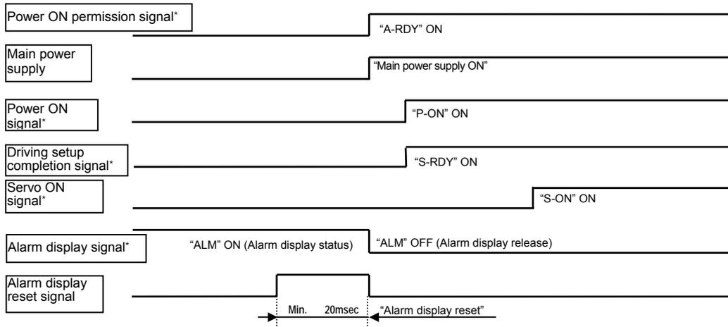
In the case of the model number: TS1B\*(50Vdc input type)
