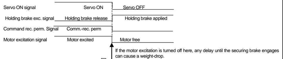
Set the delay time for the holding brake operation
