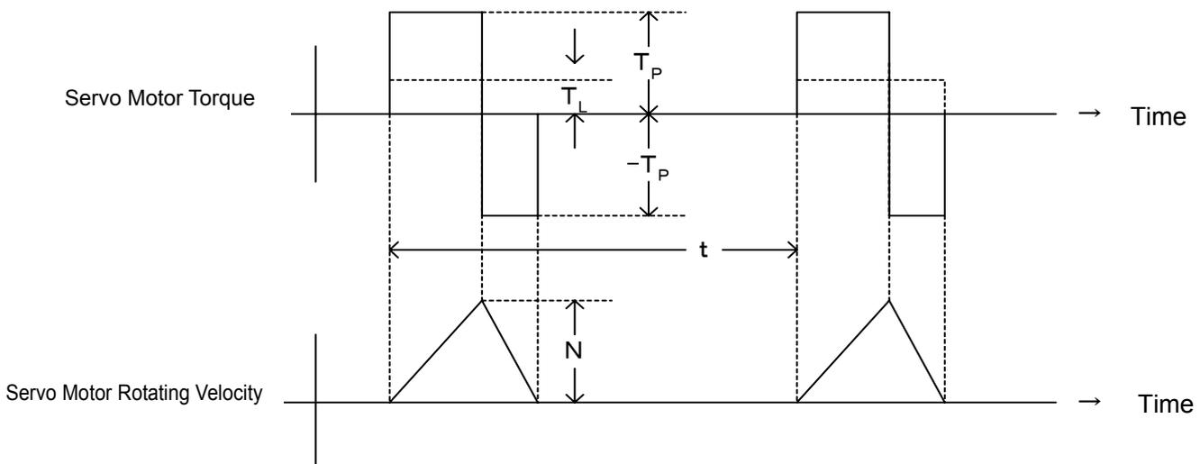
$$n = 2.86 \times 10^2 \times \frac{1}{N(J_M + J_L)} \times \frac{T_P^2 - T_L^2}{T_P^3} \times T_R^2 \quad [\text{times/min}]$$
