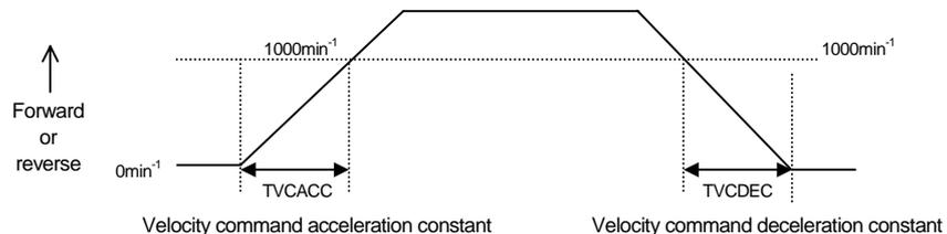
26 and 27 are commonly applicable to the following commands: Analog Velocity Command, Internal Velocity Command, and JOG Velocity Command.
