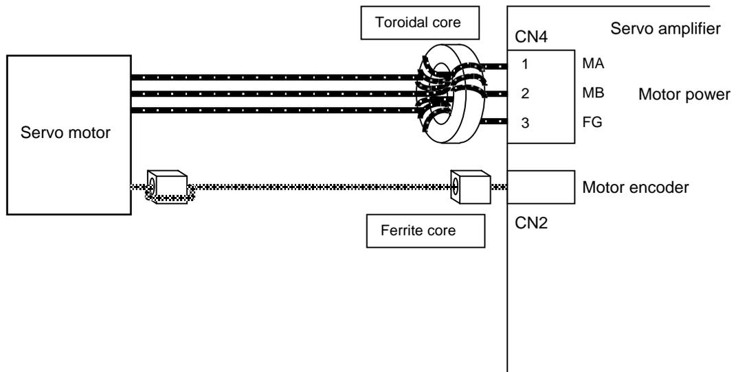
⑮ Please wrap the Toroidal core (note 3) two times around the amplifier side of the motor power line.
