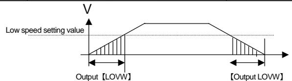
Speed Matching Width: Speed coincidence range signal is given if speed deviation reaches the set range.
