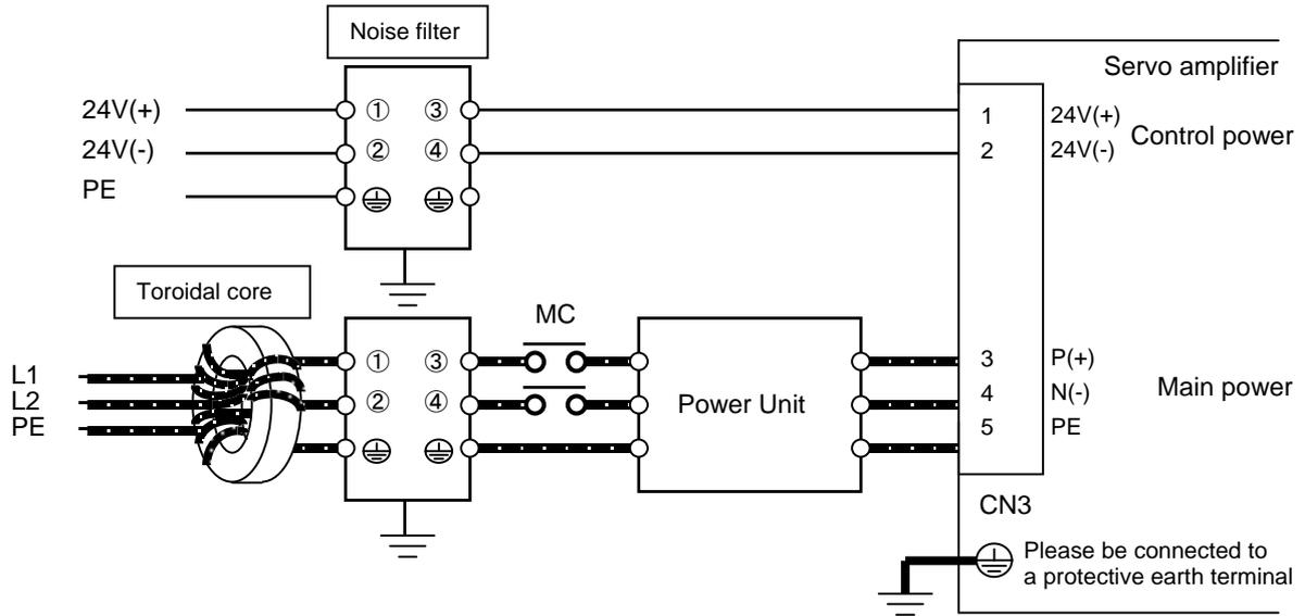
⑬ Please put a noise filter(note 1) in a power supply line. In addition, Always ground the frame of the noise filter and Install wiring by separating the primary and secondary wiring of the noise filter as much as possible.
