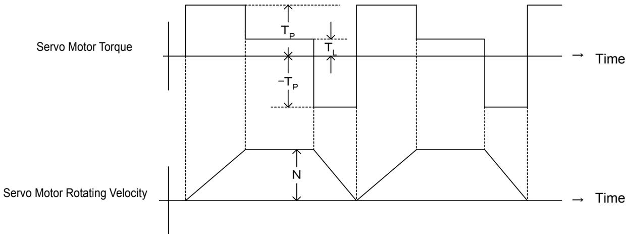
$$n = 2.86 \times 10^2 \times \frac{1}{N(J_M + J_L)} \times \frac{T_R^2 - T_L^2}{T_P} \quad [\text{times/min}]$$
