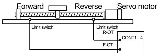
2. If the over travel function is used, select the operating conditions of “Position command input, Servo motor stop operation and Servo ON signal” in the case of over travel.
