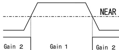
The value of gain 2 shall be set to 1.2 times the value of gain 1.
