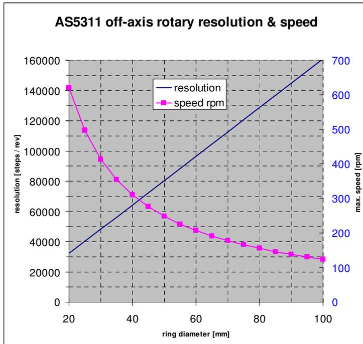
In off-axis rotary applications, very high angular resolutions are possible with the AS5311.
