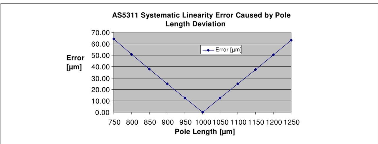
Figure 12 shows the error caused by a mismatch of pole length. Note that this error is an additional error on top of the chip-internal INL and DNL errors (see 5.5). For example, when using a multi-pole magnet with 1.2mm pole length instead of 1.0mm, the AS5311 will provide 1024 incremental steps or 4096 absolute positions over 2.4mm, but with an additional linearity error of up to 50µm.
