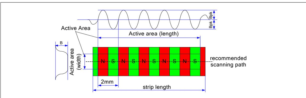
Figure 14: Alignment of magnet strip with AS5311 sensor IC
