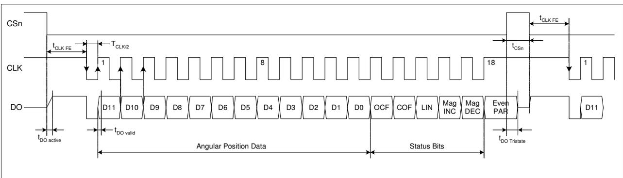
If CLK is low at the falling edge of CSn, the first 12 bits represent the magnitude information, which is proportional to the magnetic field strength. This information can be used to detect the presence and proper distance of the magnetic strip by comparing it to a known good value (depends on the magnet material and distance).
