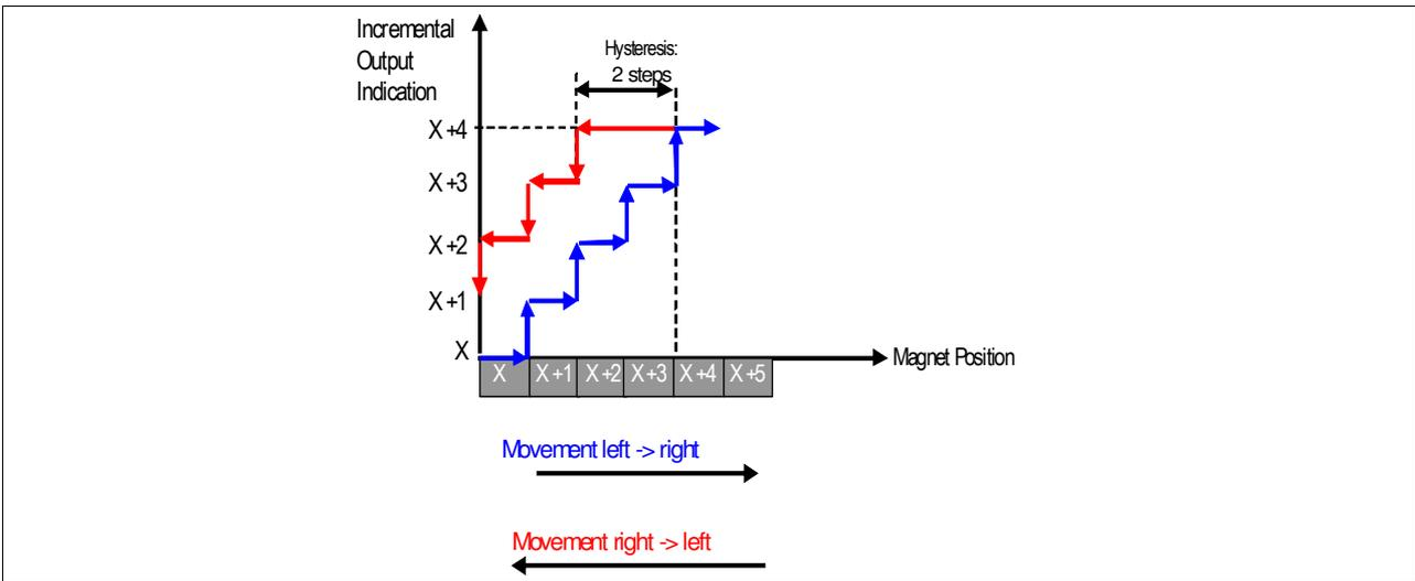
To avoid flickering incremental outputs at a stationary magnet position, a hysteresis is introduced. In case of a movement direction change, the incremental outputs have a hysteresis of 2 LSB. For constant movement directions, every magnet position change is indicated at the incremental outputs (see Figure 6). If for example the magnet moves from position „x+3“ to „x+4“, the incremental output would also indicate this position accordingly.
