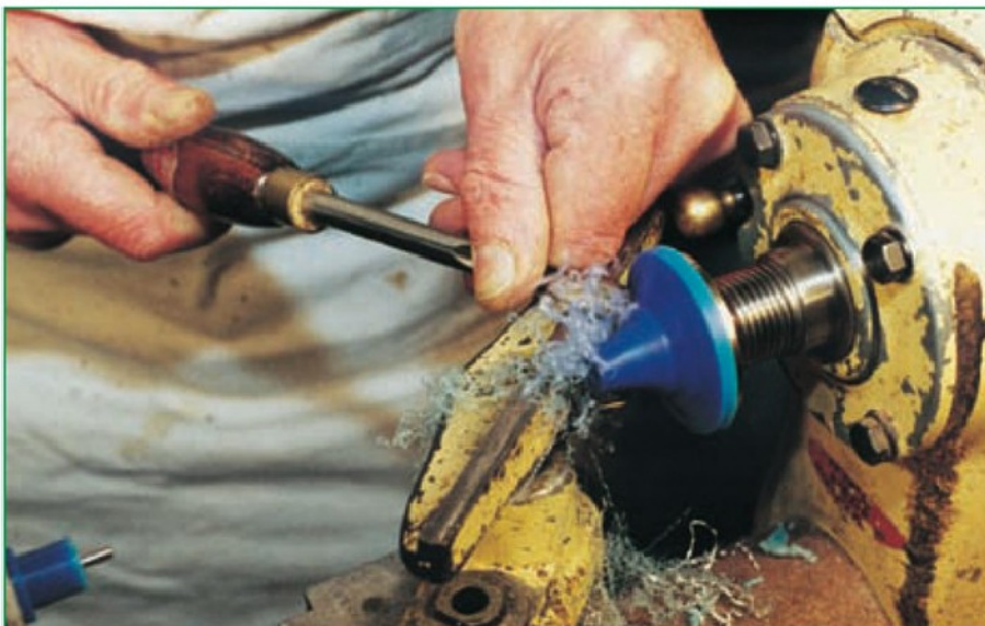
2. A mandrel being made in nylon material.
