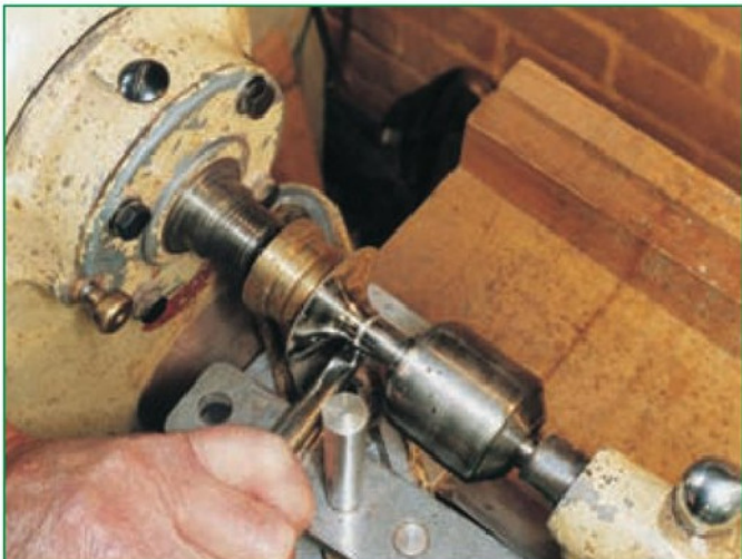
10. Ironing out the swelling using the tool beneath the work piece.
