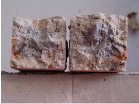
Fig. 26 Character of the geopolymers concrete after firing
