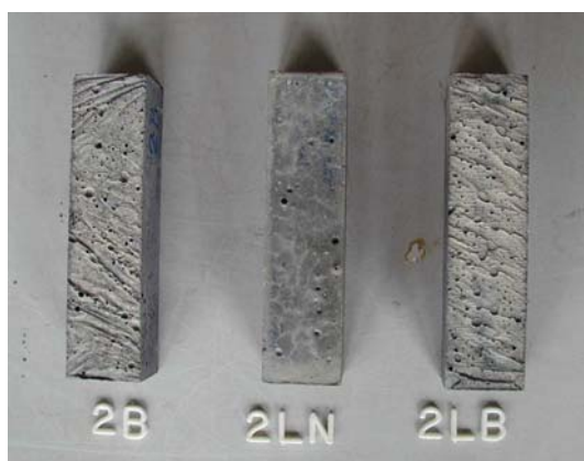
Fig. 24 A geopolymer mortar after 150 freezing cycles
