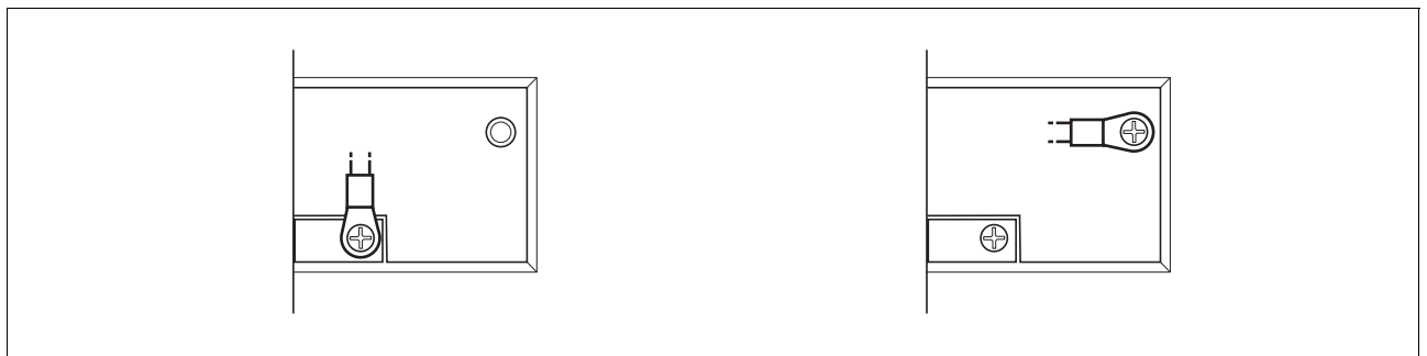
Figure 6.3 left: Y-Capacitors for the internal filter operative (standard): Y-Capacitors for the internal filter deactivated for IT networks
