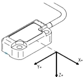
And next a 5 axes iM Smart sensor with its axis orientation:
