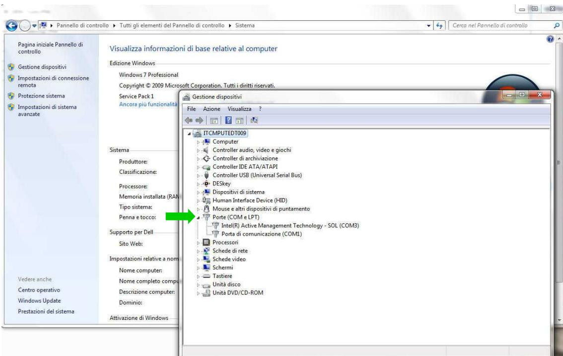
That com name must be used in the **Port** box of the HMI settings window. Now it's possible to click on **Scan** label to connect the sensor, and then close.
