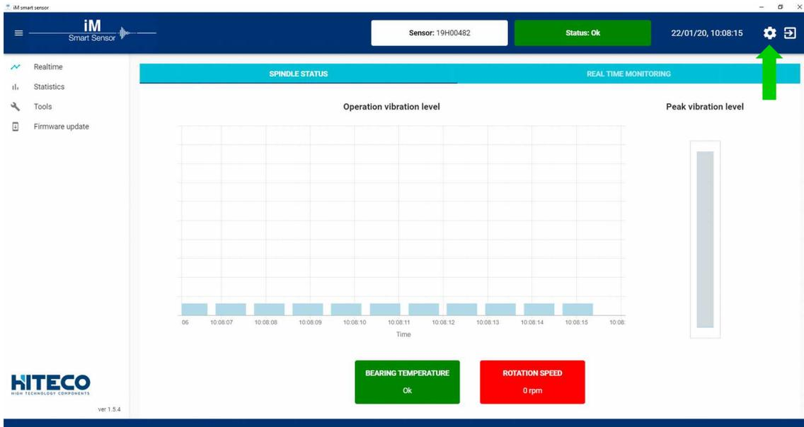
By clicking on it a new window pops up where it's possible to add to the HMI a new iM Smart Sensor. On the "+" box the HMI adds a new sensor to its interface.
