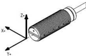
The 3 axes iM Smart Sensor is located on the front side of the spindle and connected inside the electrical box. The 5 axes sensor is located inside the shell and connected through signal cables of the spindle. Due to rs485 protocol the iM Smart Sensor needs a proper serial bus converter (rs485 to usb) and a pc as user side interface.
