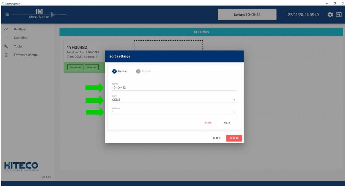
After the installation of the Rs485 to usb converter with its drivers on windows, it's possible to know the assigned com port by going in Windows control panel and look to the system tab, device manager. Here, after the rs485-usb converter has been correctly installed, a new COM port will appear under the COM ports folder.
