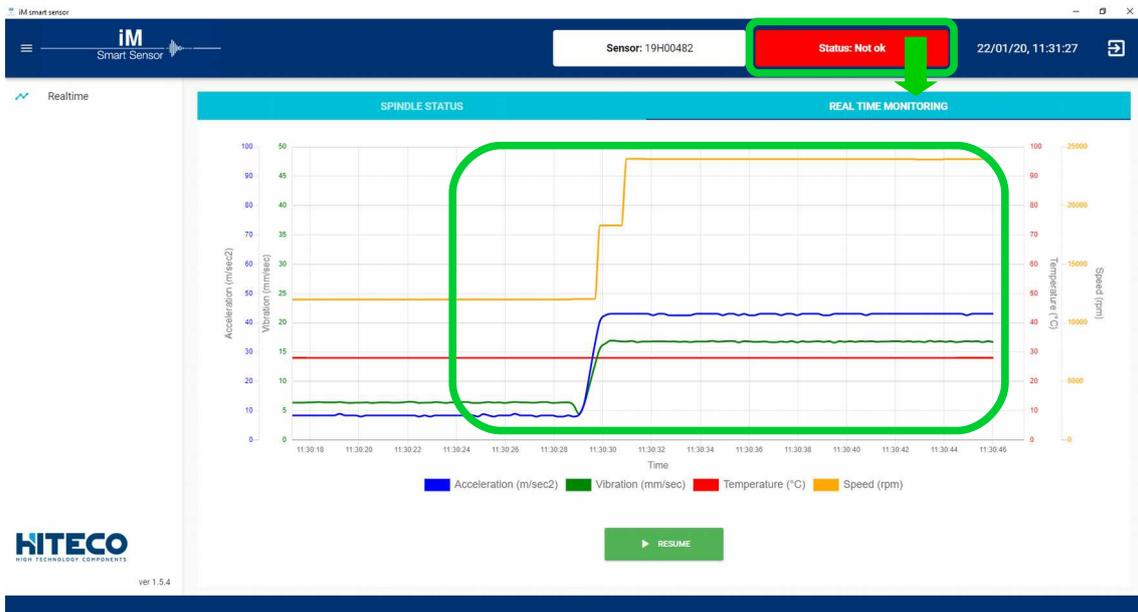
By decreasing of vibration level the **Spindle status** shows decreasing bars with colors that turn from red to grey. Also the **Status button** turns from red to green, signalling that the spindle working conditions now are safe.
