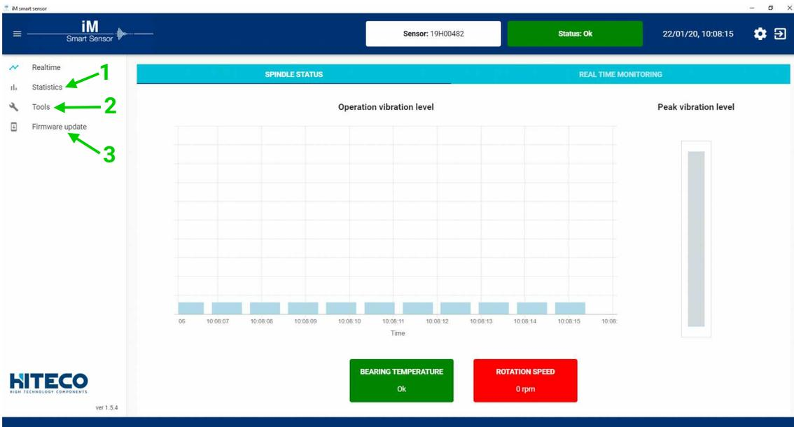
By clicking on **Statistics** label the HMI shows 3 new labels that categorizes the available time-accumulated physical quantities measured by iM Smart Sensor (speed, vibration speed, temperature).
