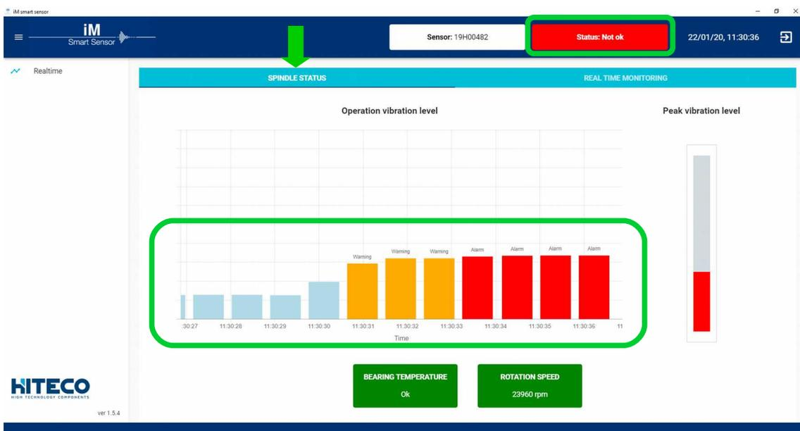
The same vibration level increase is showed in the **Real time monitoring** tab by time varying magnitudes. Even in this case an event of vibration level increase turns in red the **Status button** but here the HMI shows the values sampled by iM Smart Sensor.
