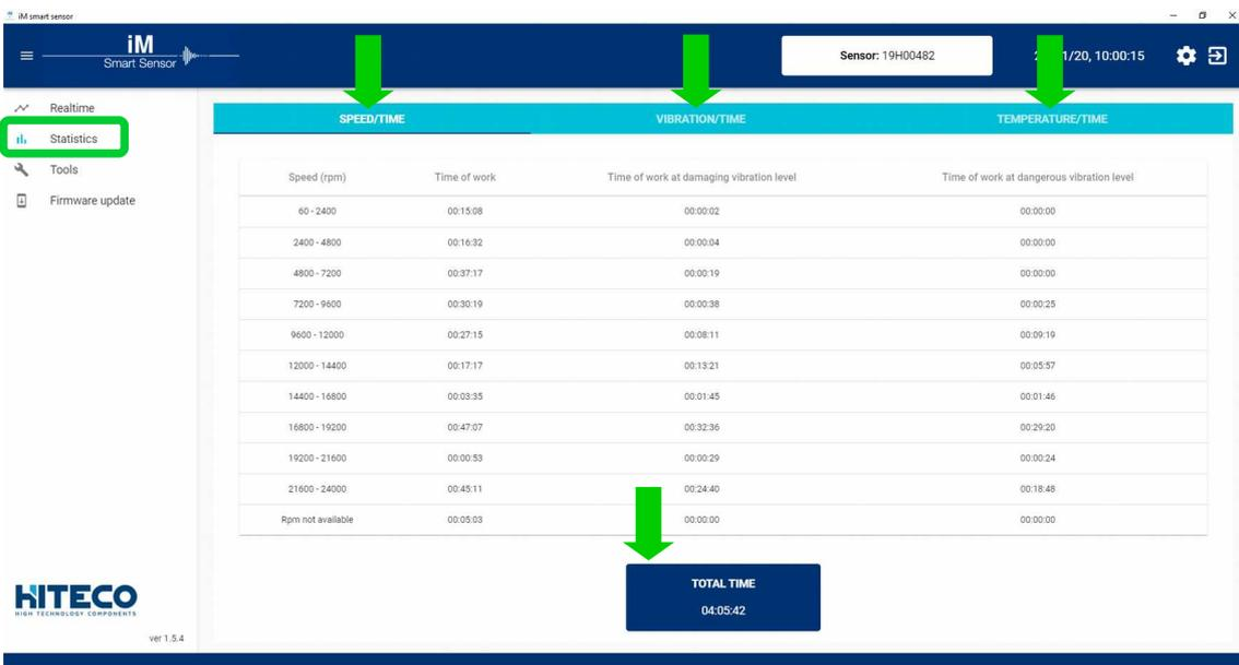
Also a total working time counter is present in the bottom of the screen.
