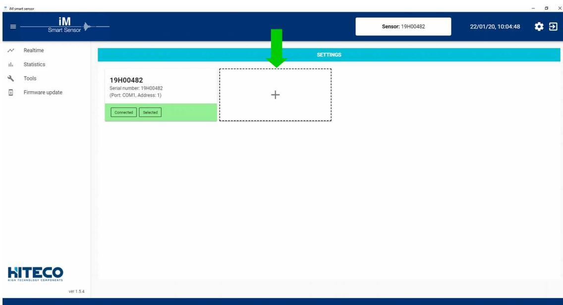
A new window pops out where it's possible to configure the communication settings of the sensor such as name of the sensor (as default the spindle serial number), Com port (defined by windows settings and type of rs485-usb converter) and address (as default set to 1). For multiple sensor installation it must be used the address 1 to communicate the first time with each sensor, before assigning the desired modbus address.
