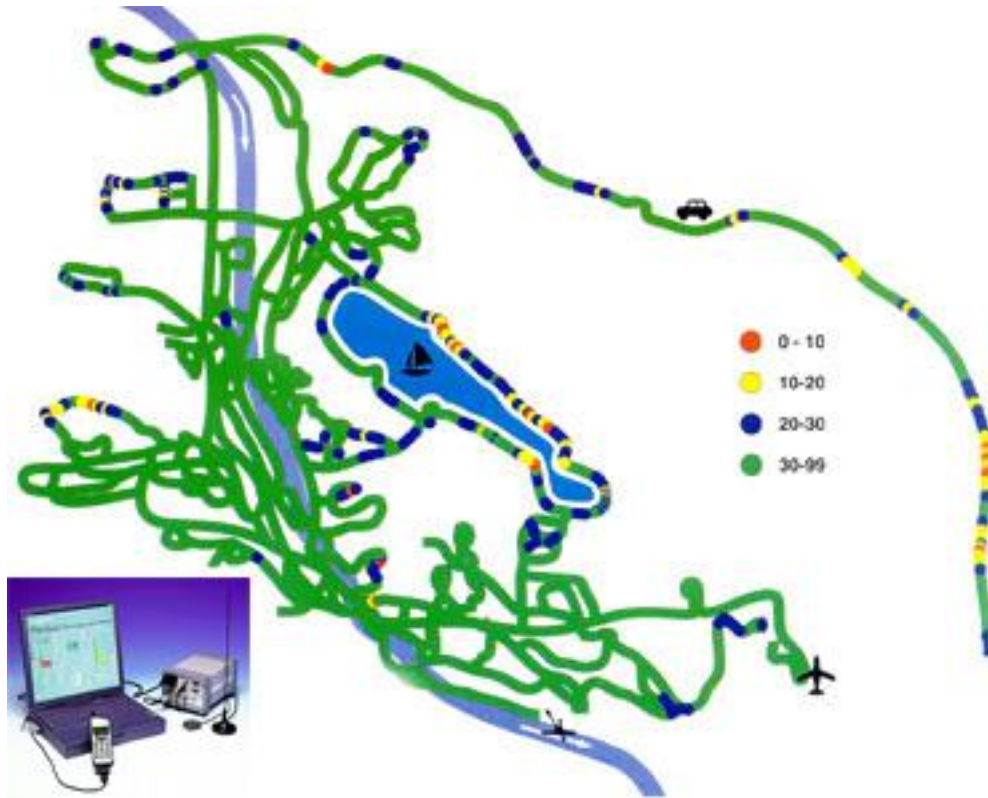
Figure 16: map of Drive Test - The method of GSM signal testing
