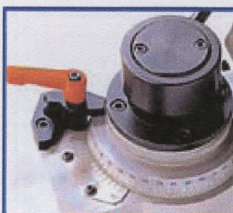
Rapid cross movement with hand lever.
