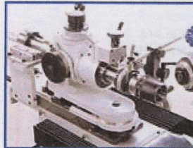
When grinding with the support finger, the control roller is lifted and the work spindle is free in both axial and radial directions.
