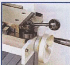
Rapid cross movement with hand lever.
