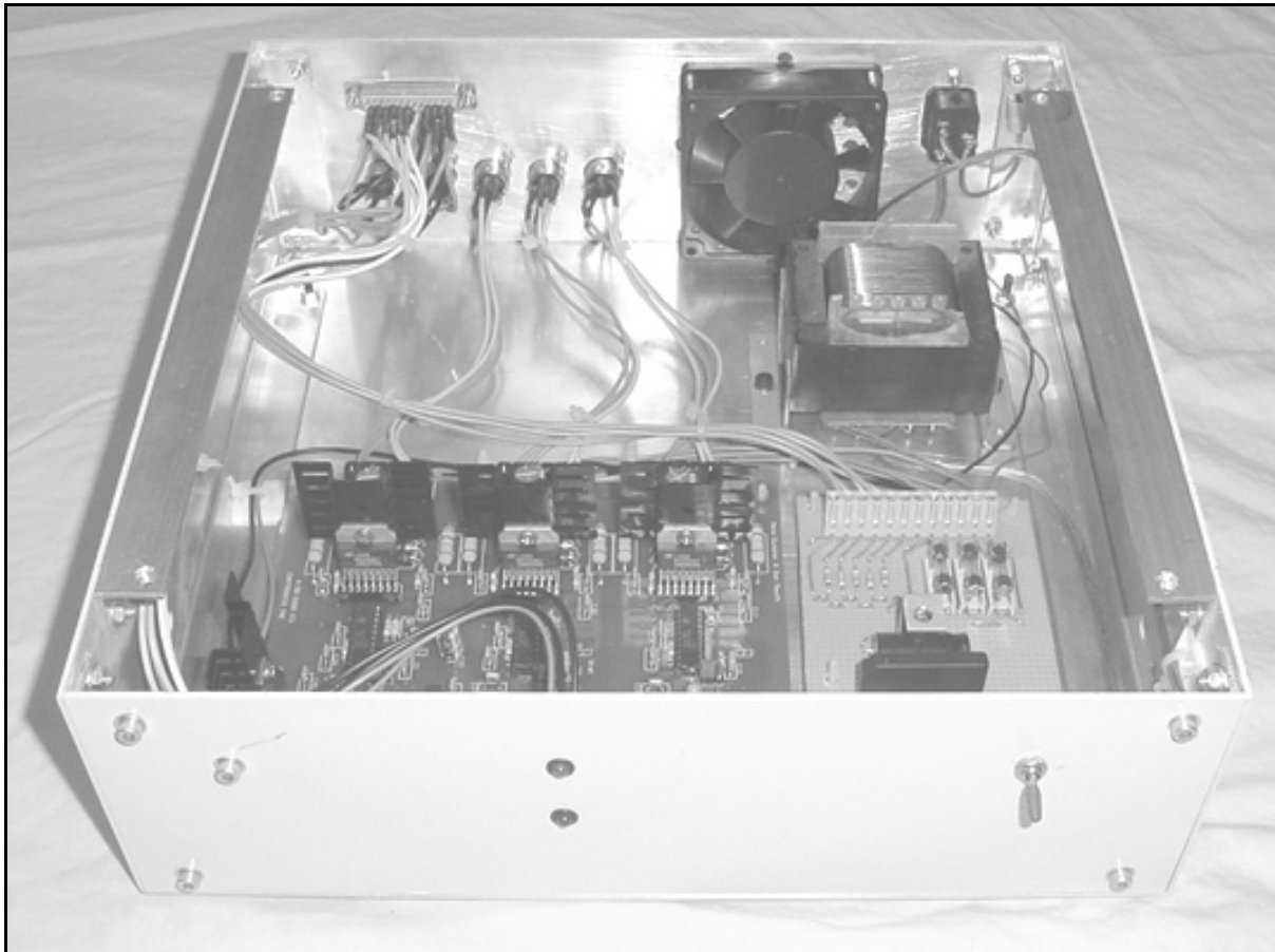
Fig.40 Completed Driver Circuit & Power Supply
