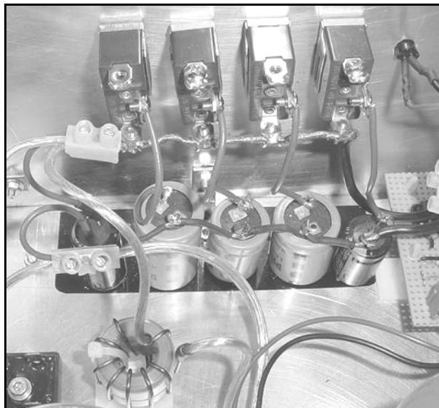
Fig.33 EDM Capacitors
