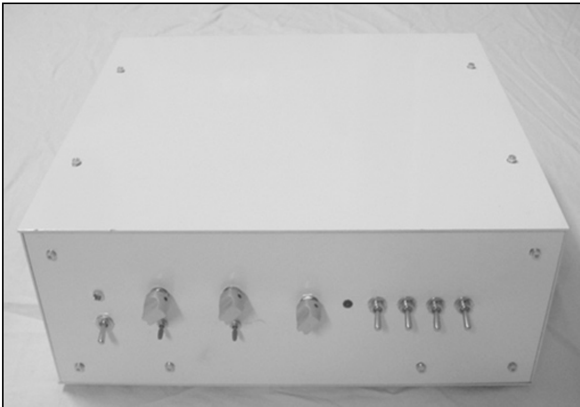
Fig.34 The Completed EDM Circuit Housing
