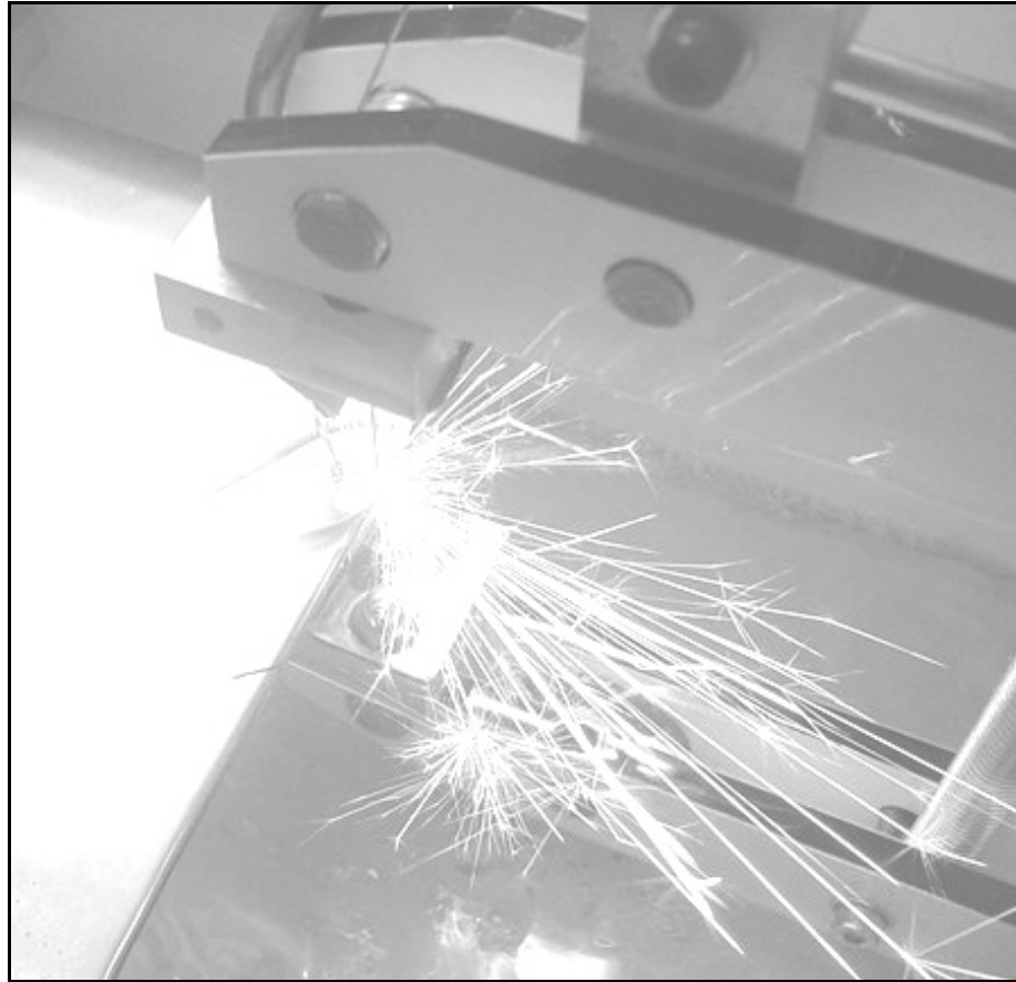
Fig.1 Wire-EDM in Action
