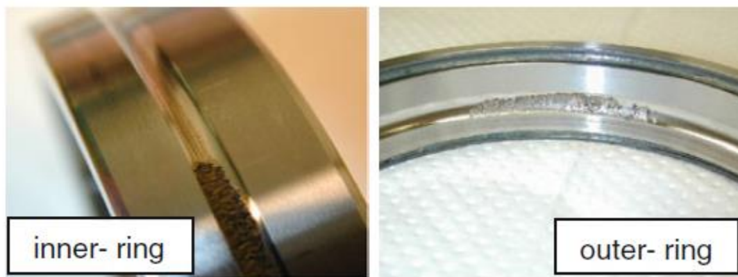
Figure 60 Failure on the inner and outer ring after disassembling spindle in (Neuebauer, et al., 2011)
