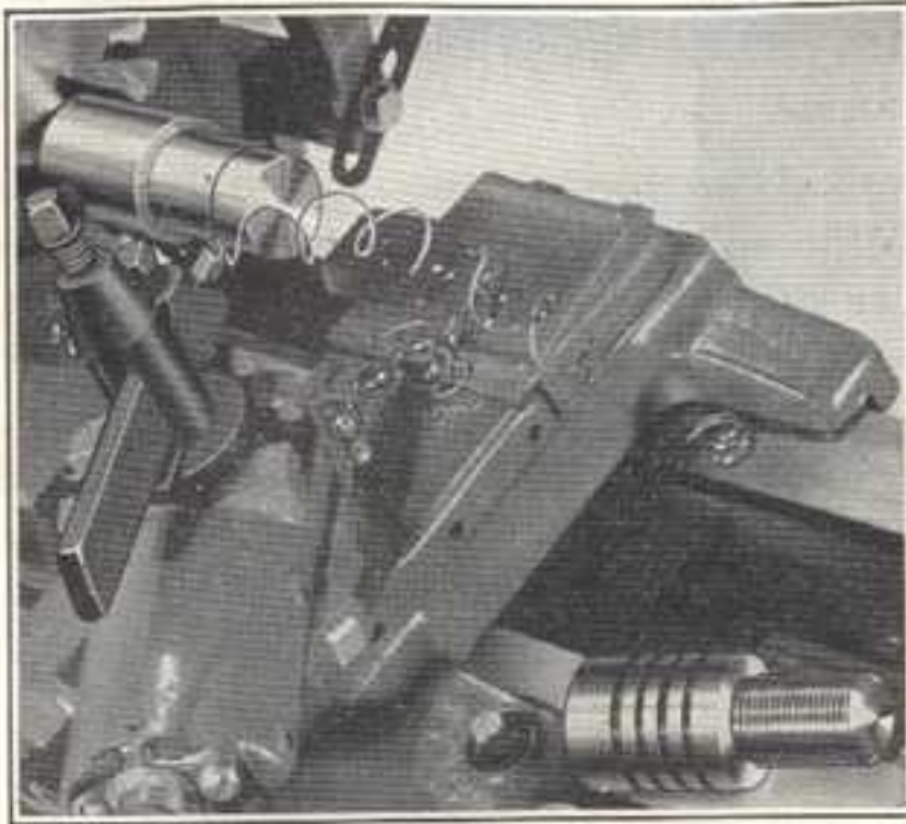
FIG. 64 Machining a solid copper electrode on the lathe. A finished electrode is also shown.
