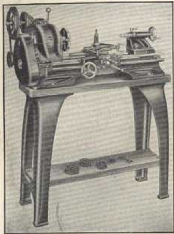
FIG. 2 (Left) Lathe on floor stand. This type of mounting provides a rigid support and avoids imperfections of many shop benches.
