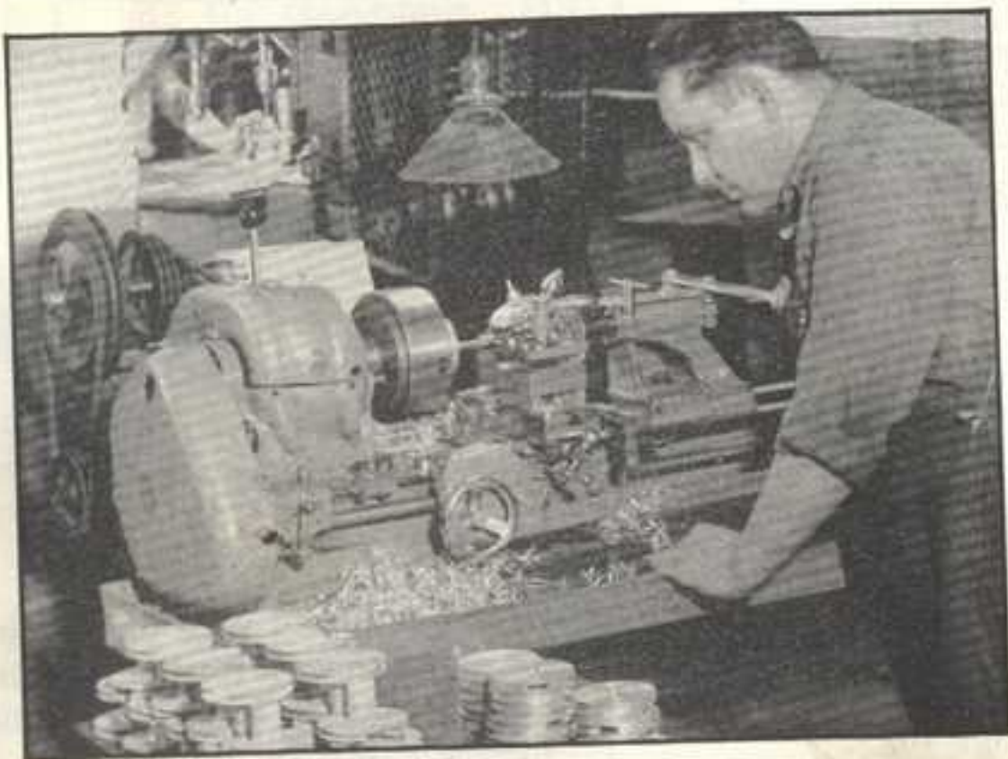
FIG. 12 Timken-equipped lathe handling continuous high speed production operations.
