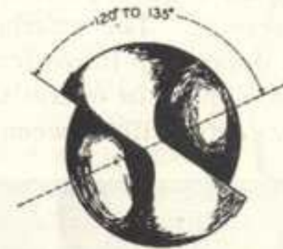
FIG. 106B End view of drill point showing proper angle be- tween point and lip.
