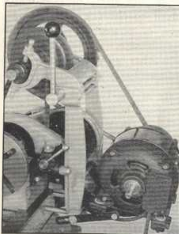
FIG. 14 (Right) Support bracket for horizontal countershaft is mounted on the lathe bench or stand.
