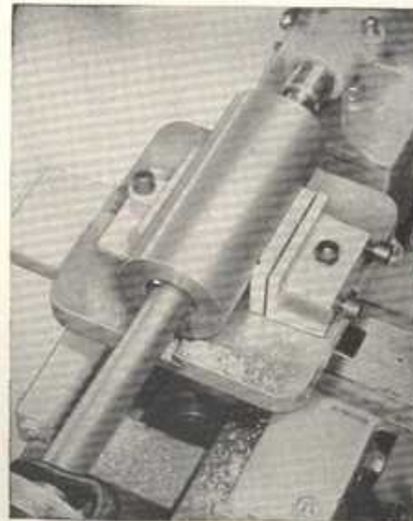
FIG. 121 Boring a small grinder spindle bearing housing held in the boring table and vise.
