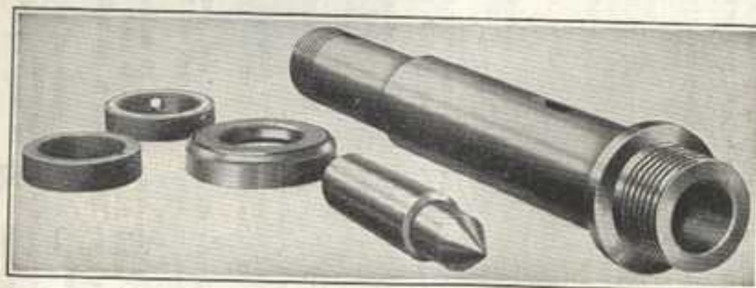
FIG. 6 Headstock Spindle, Take-up Nut and Collar, Ball Thrust Bearing, Center and Sleeve.
