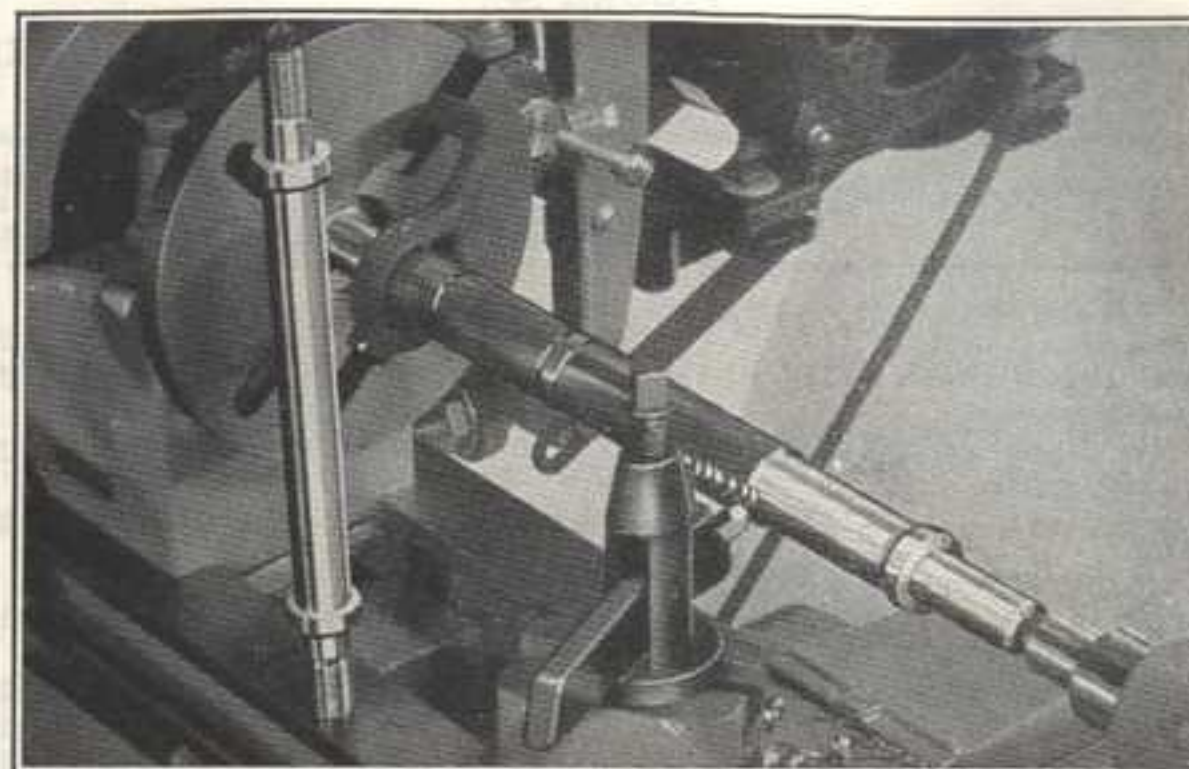
FIG. 58 A small alloy steel grinder shaft being turned in the lathe. The finished shaft is also shown. Note the grooves made by the cut-off tool for blocking out the work for roughing (see page 162).
