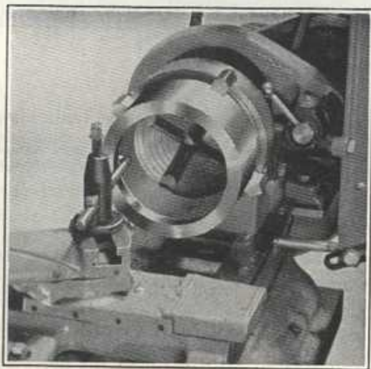
FIG. 117 Boring the inside of a large steel bushing. Note high-speed boring tool mounted directly in tool post for maximum rigidity.
