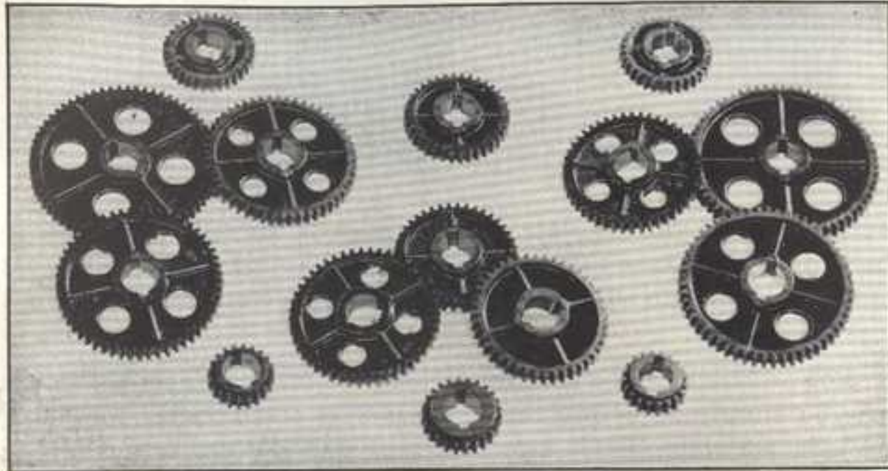
FIG. 29 Threading Gears.
