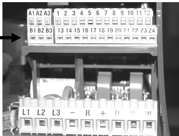
Figure 5.1.1: Accessing the power and control terminals
