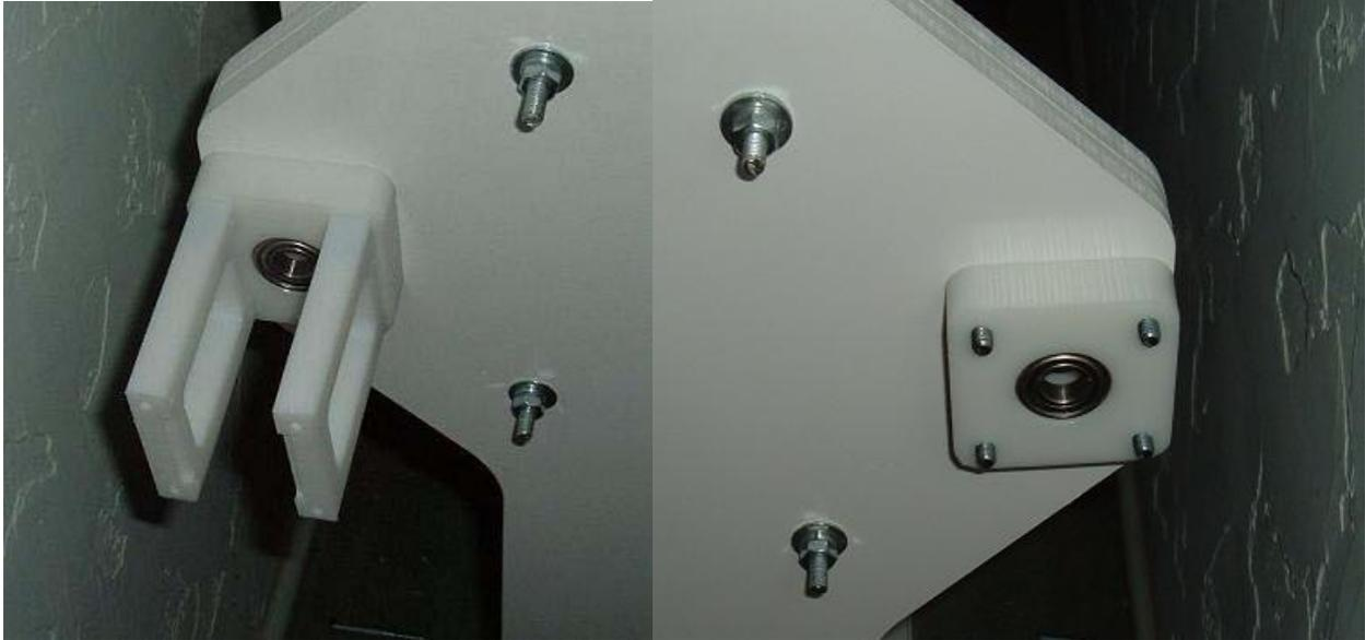
You will notice that the Motor mount walls will be taped on one end with 1 /4" threads and the other with 10-24 screw threads. And three of the bearing holders will have 1/4" Holes drilled in them and three will have 1/4" tap threads (one of each for the all axis). To install the bearing holder and motor mount use:
