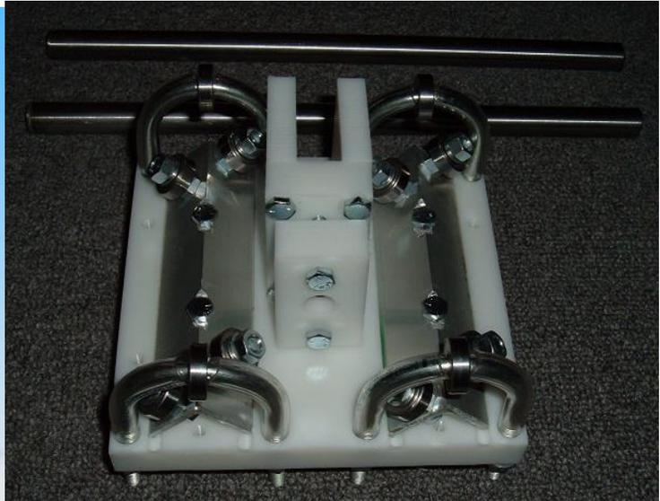
Place the bottom larger piece of the z-axis anti-backlash nut (this one is slightly different from the other axis with the bolt pattern) on top of the two z-axis anti-backlash nut support walls (1/2" thick HDPE) both ends should be flush, then drill and tap the walls and bolt bottom of anti-backlash nut to them with:
