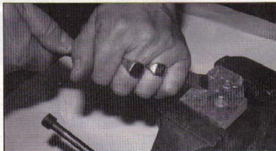
The flat scraper shown in action.
