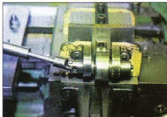
5. The cam bears on a roller fitted to the end of the tool holder.
