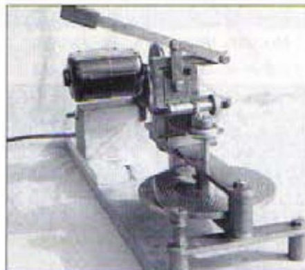
2. A view showing the vertical slide and the division plate with its detente
