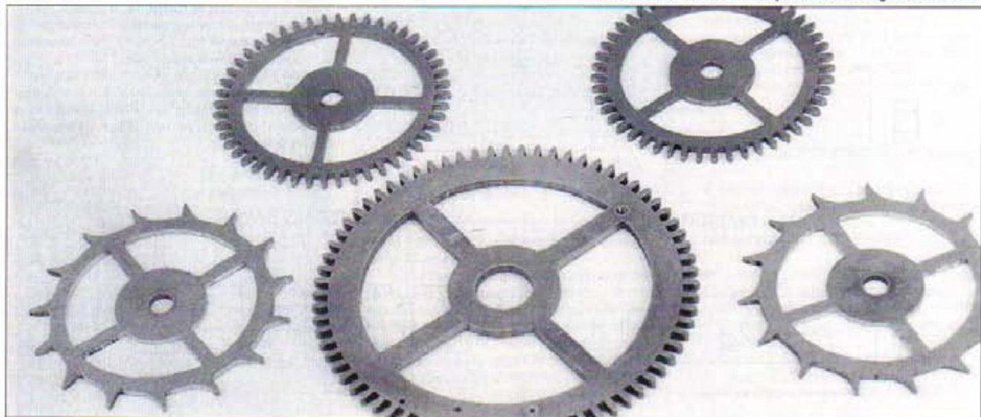
6. A selection of wheels produced using the machine
