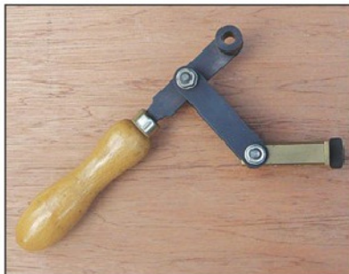
Photo 9. The actuating handle assembly.
