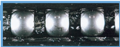
Detail view of the ball cage
