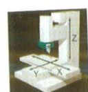
BK machines have three powered linear axes (X, Y, Z).
