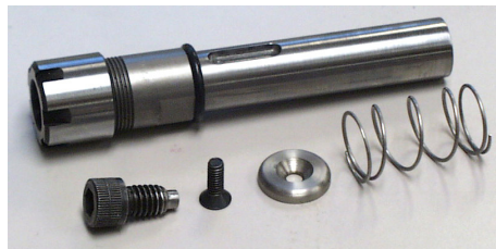
The tap holder will fit in all of the tooling bars with a 5/8" bore.
