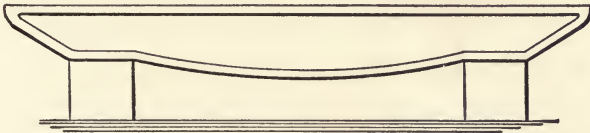
FIG. 31. — The Parabolic Design of a Lathe Bed.
