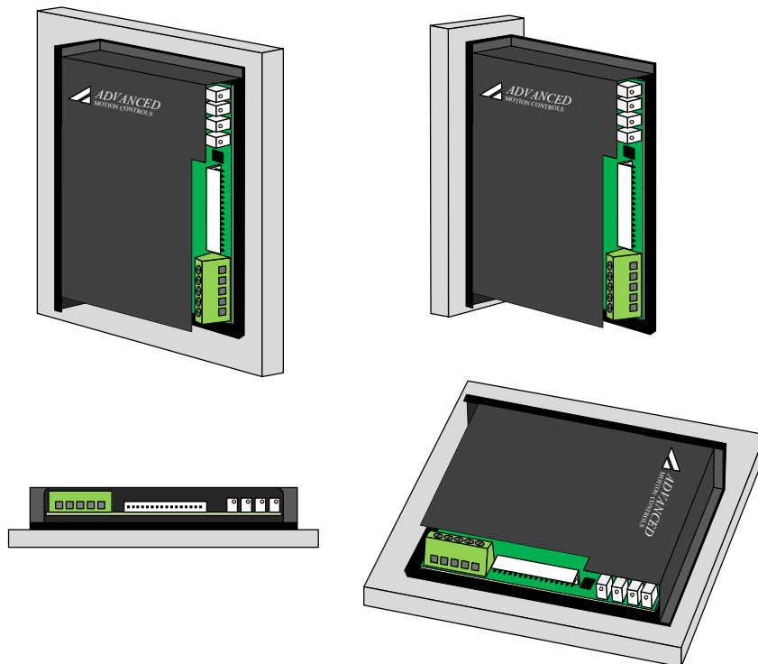
FIGURE 3.17 Analog Servo Drives Mounting Options
