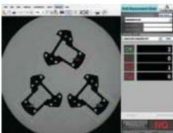
Judgements can be made at a glance thanks to the OK/NG display.
