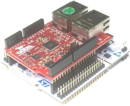
**Fig. 5** The EasyCAT Shield on an STM32 NUCLEO board
